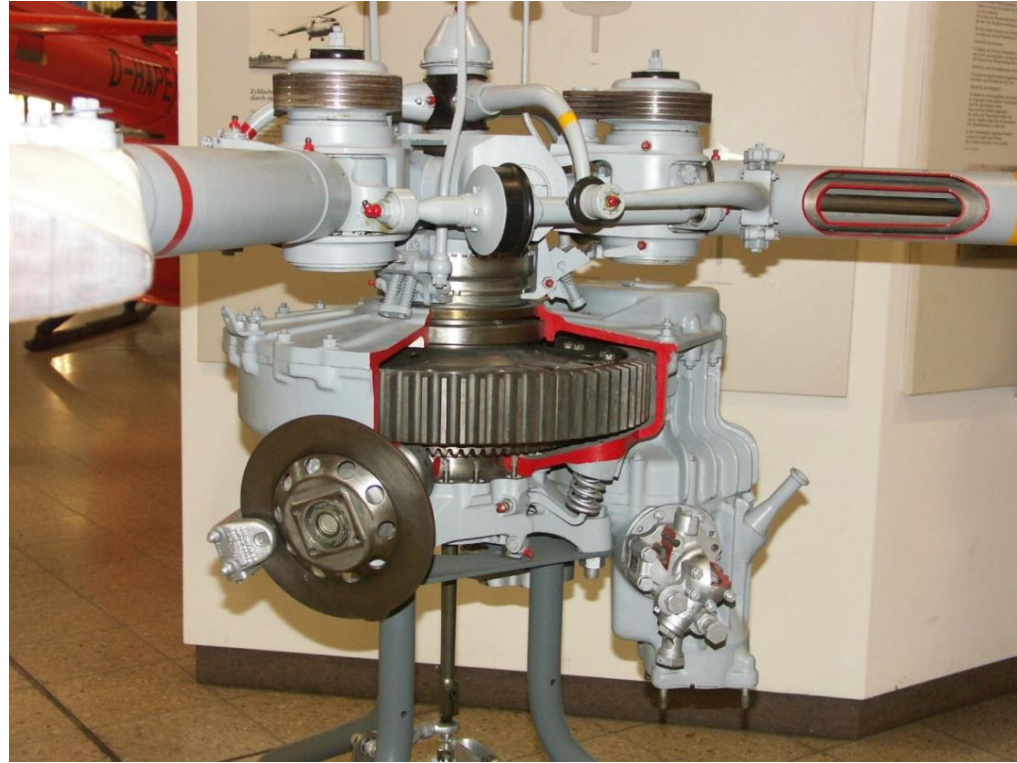
Bristol 171 Sycamore helicopter main gear box and rotor head. Source: Wikimedia Commons.
