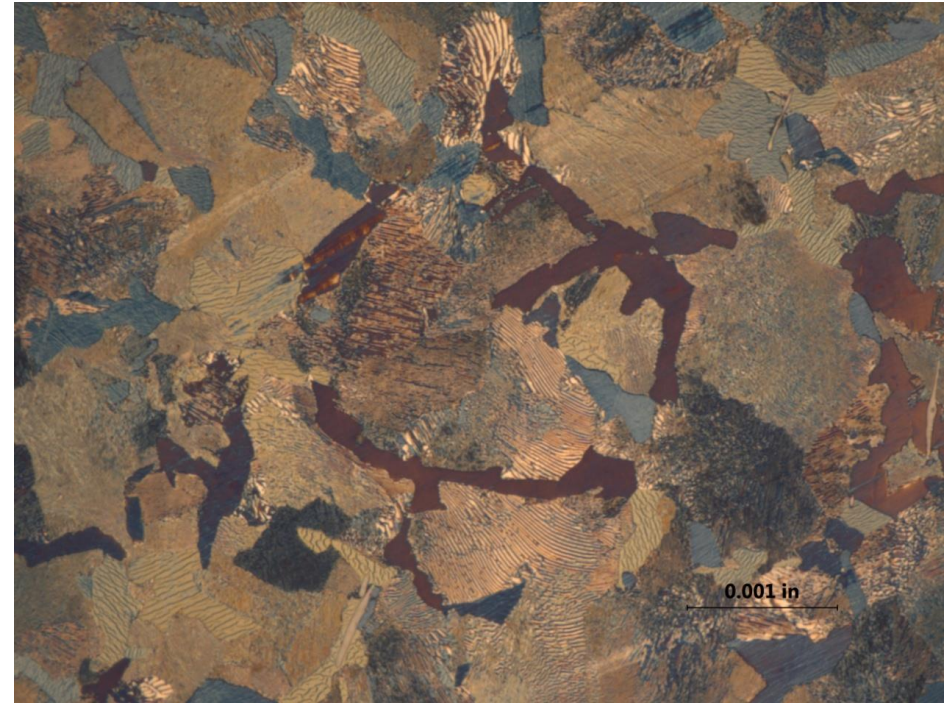
AISI 1050 steel microstructure prepared with color tint etching. The ferrite appears red and blue in this image. This sample was etched in Klemm's reagent. Original magnification 1000X.
