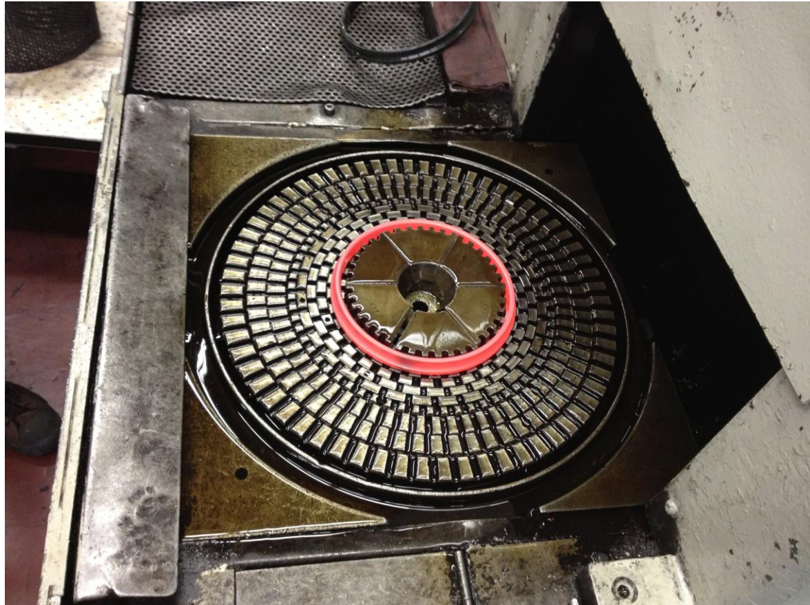
Lower expanding segmental die tooling for an industrial bearing ring.
