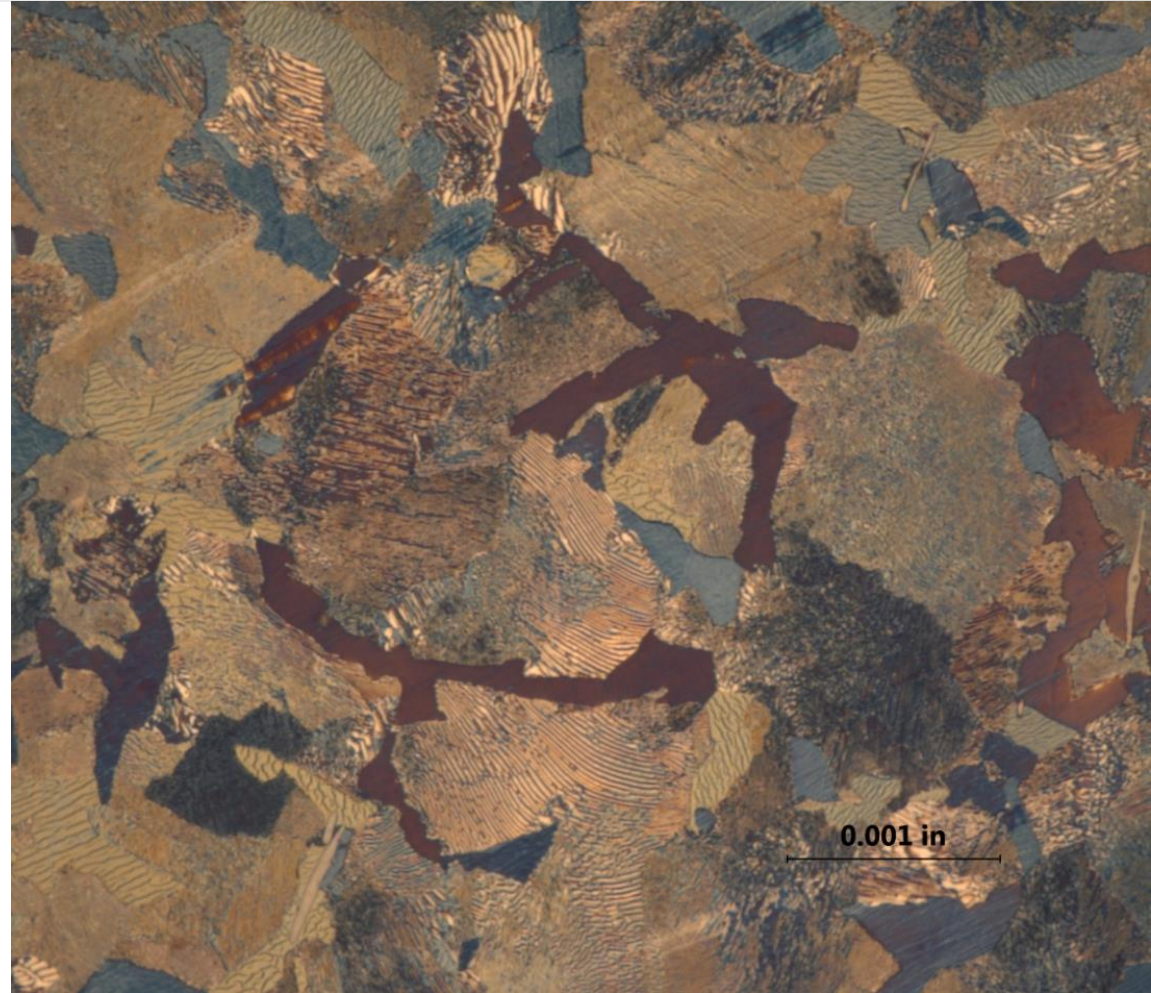
AISI 1050 steel microstructure prepared with color tint etching. The ferrite appears red and blue in this image. This sample was etched in Klemm's reagent. Original magnification 1000X.
