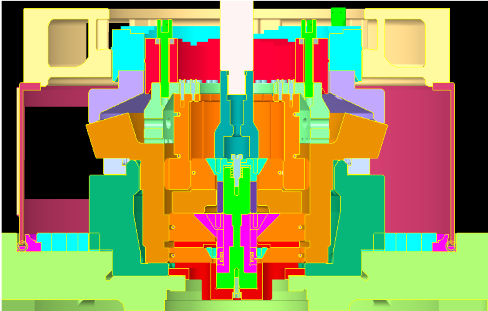
Stacked expanding die tooling set-up. The quenched part is colored orange.
