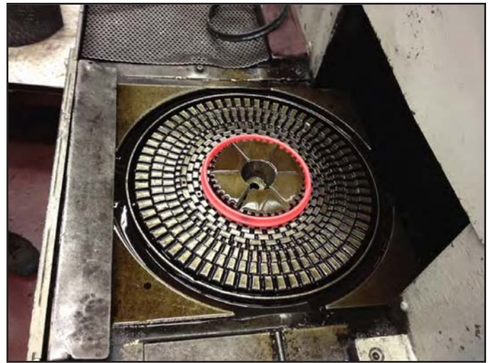
Figure 3 Hot bearing race positioned on the lower die assembly of a quenching machine just before it is retracted into the machine for quenching. Note the segmented die tooling and individual slotted rings. The slotted rings may be independently adjusted to control the flow of oil over the part being quenched.
